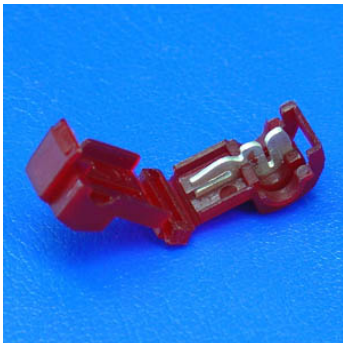
K951 Main cable cross section: 0,65-1,0 Tap cable cross section: 0,5-1,0mm 2
