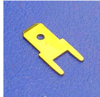
30-315 Tab: 4.75x0.5 Dimensions mm W: 6.3 Dimensions mm L: 12.7 Material: Brass
