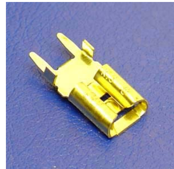
30-323 Tab: 6.35x0.8 Dimensions mm W: 7.5 Dimensions mm L: 16.8 Material: Brass
