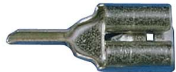
3-7566 Tab: 6.3x0.8 Dimensions mm W: 7.5 Dimensions mm L: 18.0 Material: Tinned Brass
