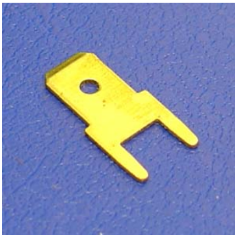
30-321 Tab: 6.35x0.8 Dimensions mm W: 7.9 Dimensions mm L: 14.0 Material: Brass
