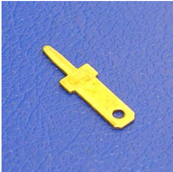
30-313 Tab: 2.8x0.5 Dimensions mm W: 4 Dimensions mm L: 13.8 Material: Brass
