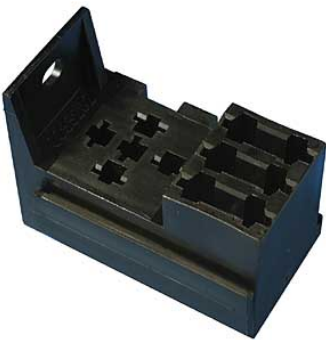
Art number RELF-1 Remark: 3-way fusebox plus one position for mini-relays or flasher unit. Terminals for blade fuse section: 30-799 1.0-2.5 mm 2 30-800 4.0-6.0 mm 2 Terminals for relay section: 3-2922 = 0.5 - 1.0 mm 2 3-2922/1 : 1.0 - 2.5 mm 2 3-2922/2 : 2.5 - 6.0 mm 2
