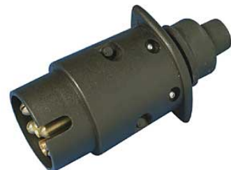
PP7 : Hinged plug 7 pin, 12 Volt, Din72577/ISO1724. Hygrade thermoplastic, vertically divided, locking device nut cap with grommet, cable holder & stopper
