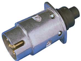
PP7M : Plug 7 pin, 12 Volt, DIN72577 DIN72577/ISO1724-12N. Hygrade aluminium vertically divided, easy grip ridges.
