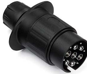
PP13W : WeST Connector as per ISO 11446. Current carrying capacity: 25 A at 12 V. Screw connections.
