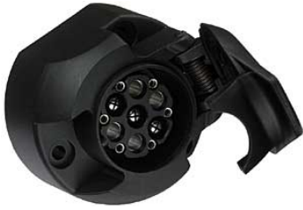
PS13R : WeST Socket as per ISO 11446. Incl. rubber seal. Current carrying capacity: 25 A. at 12 V. With micro switch-off for rear fog light-Screw connections.
