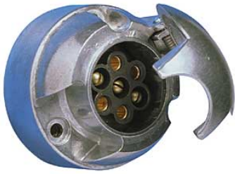
PS7M : Socket 7 pin, 12 Volt, DIN72577/ISO1724-12N. Removable terminal block. Hygrade aluminium
